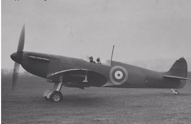
Early built Spitfire Mk.I, with two-blade wooden Weybridge propeller, early style antenna mast, early style Pitot tube, with no armor, no gun heating, having flat canopy and iron sights.
